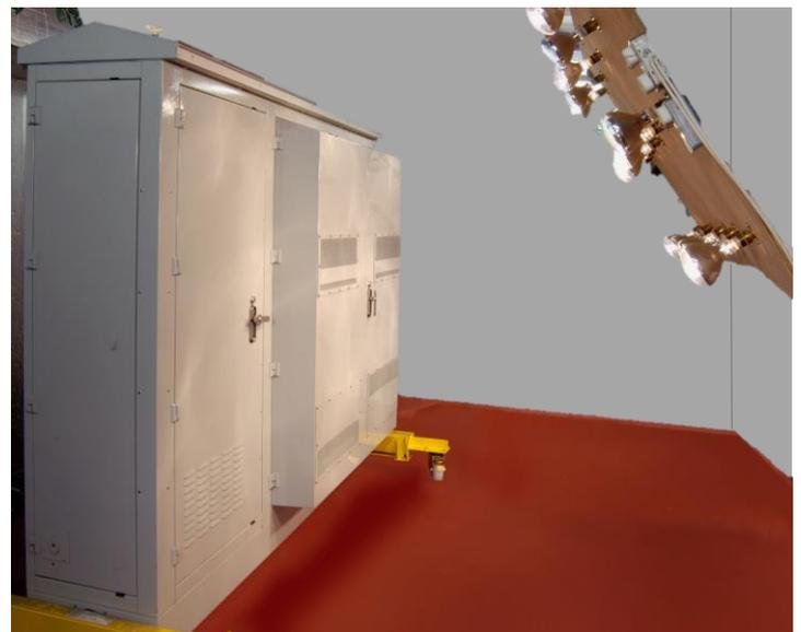
Chamber capable of maintaining air temperatures above the local ambient up-to a maximum 60°C with a solar gain of 1.1kW/m<sup>2</sup>
